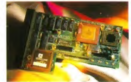
A 50 Mhz 68030 ensures the the 1230XA doesn't get left behind in the speed trials.
